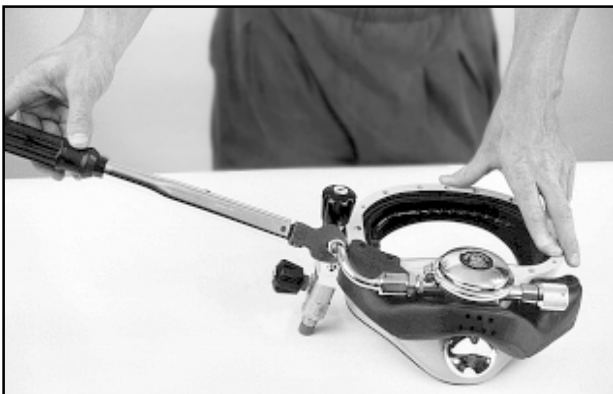
Fig. 6.43 Always start removal of the bent tube at the side block end of the tube.
