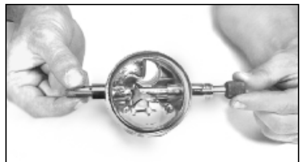
Fig. 6.63 Use the DSI socket wrench to turn the nut on the inlet valve.
