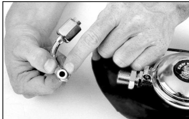
Fig. 6.44 Inspect the Teflon O-ring on the bent tube and replace if needed.
