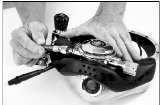
Fig. 6.42 Replacing an "A" regulator hose.
