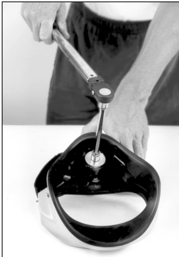
Fig. 6.46 You will probably need to loosen the regulator mount nut to position the bent tube.
