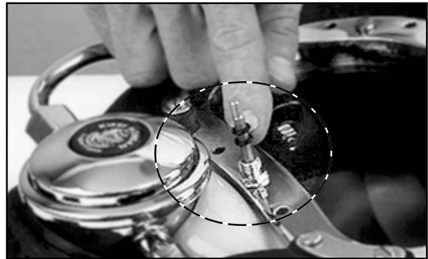
Fig. 6.49 Be sure to reinstall the nose block device O-rings.
