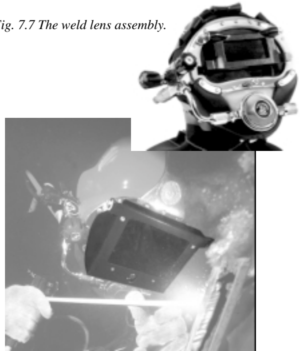
Fig. 7.8 The weld shield assembly.
