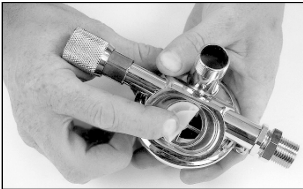
Fig. 6.52 Inspecting the regulator exhaust.
