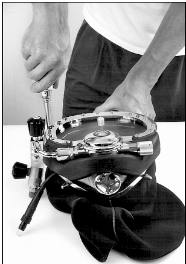
Fig. 6.54 Be sure to tighten the screws that hold the whisker and port to the proper torque settings. The correct setting is 12 inch pounds (13 kg cm). See Appendix 1 for a complete listing of torque specifications.
