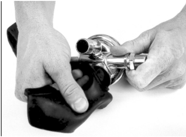
Fig. 6.51 Removing the whisker from the regulator.
