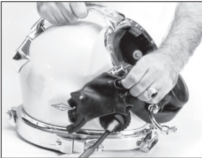
Position the shroud over the side block.
