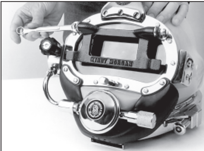
Tighten the weld lens assembly.
