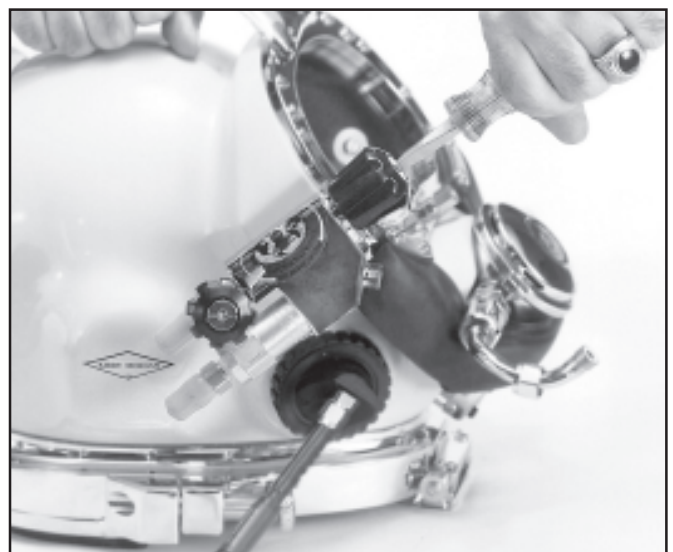
Remove the free flow knob.
