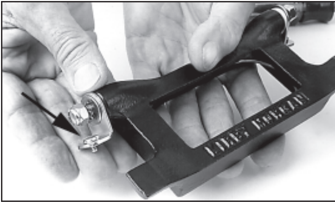
Install the screws through the mount ears.
