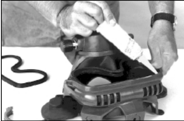
Apply silicone grease to the mask seal.
