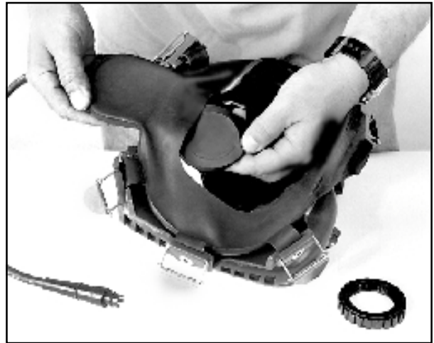
Remove the earphone assembly.
