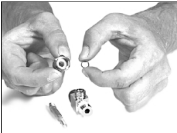
Inspect the packing and washer
