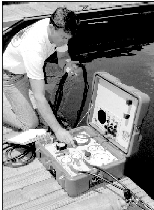
Fig. 10 DCS-2A operator taking a reading with the pneumo knob. The knob should be turned very slowly.
