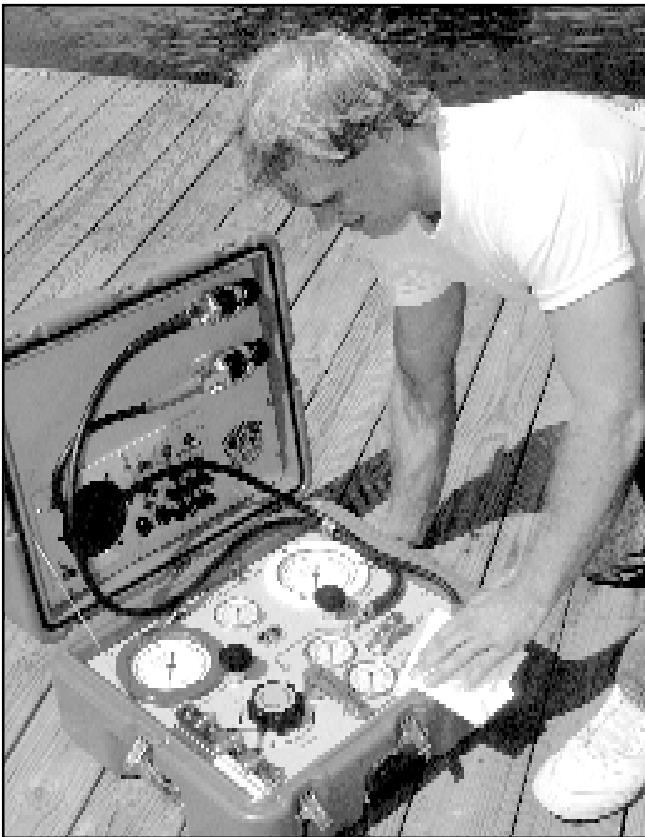
Fig 12 After each use the case, interior panels and high pressure hoses should be wiped down with a rag which has a small amount of Armor-All. Never spray cleaners directly on the DCS-2A.
