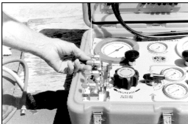
Fig. 11 All of the outlet fittings on the DCS-2A must be capped prior to storage.
